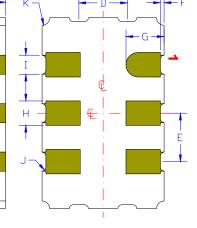
Contacts: Gold 11.8 to 39.4 μinches (0.3 to 1.0μm) over Nickel 50 to 350 μinches (1.27 to 8.89 μm) <sup>1</sup> Typical dimensions
